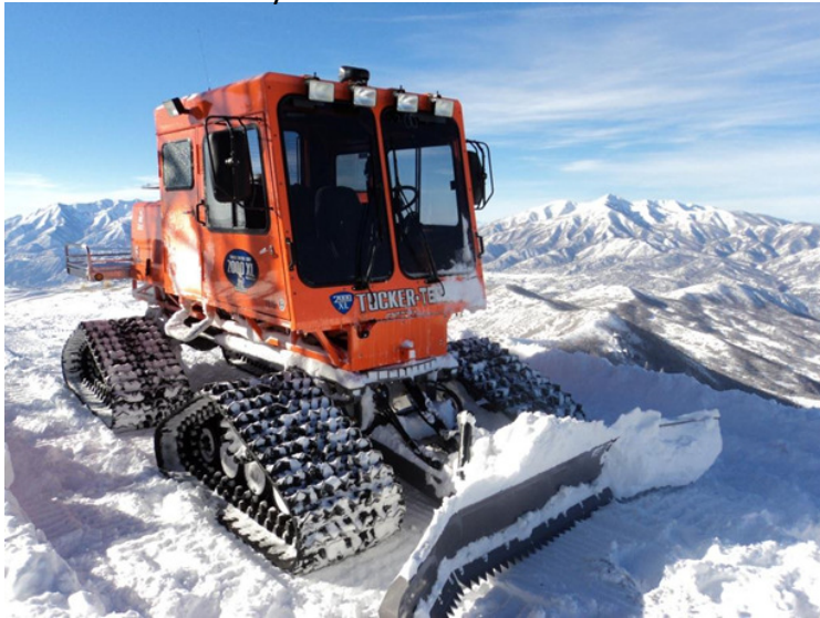
(2) Each 2013 2000BXL W/8' 6-Way Blade 26" All Rubber Terra-Tracks
