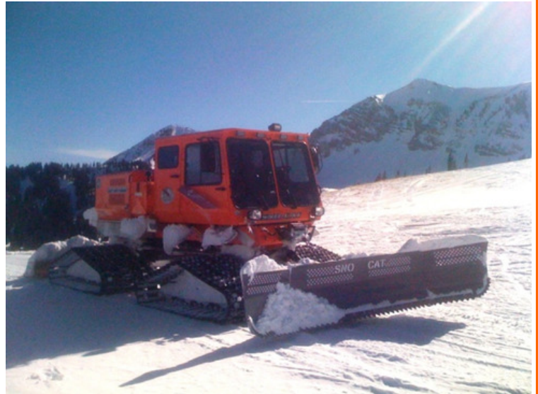
2013 2000E 5-Pass, 12-Way Blade / & Tiller 38" Tucker Rubber Bar Tracks
