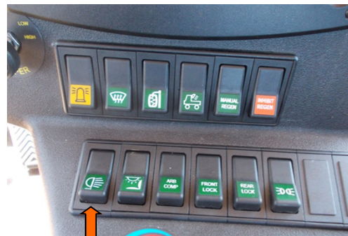
NEW ROCKER SWITCH FOR LOW BEAM LIGHTS
