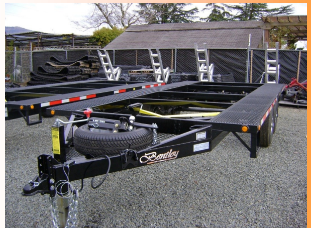
10k Demo Transport Trailer Empty Weight 1780 lbs. Dual Axles w/ Electric Brakes Used Two Seasons
