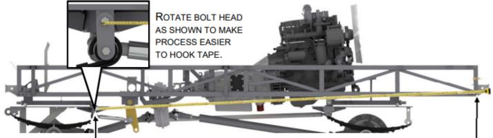
MEASUREMENT POINTS (BELOW) ARE DESIGNED TO ALIGN THE REAR FIFTH WHEEL. PULL A TAPE MEASURE FROM THE FRONT FIFTH WHEEL'S FIXED POSITION SPRING HANGER TOP BOLT, TO THE LOWER CORNER THE FRAME RAIL AT THE FRONT OF THE FRAME. REPEAT THE PROCESS ABOVE.
